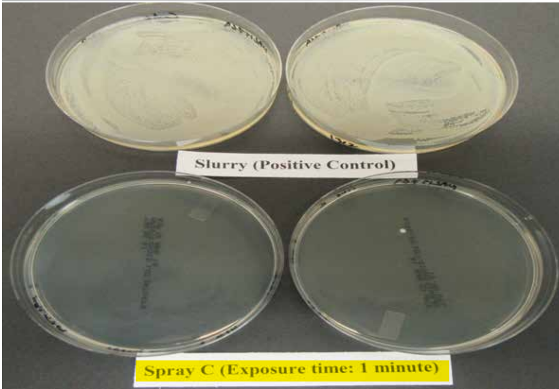
Fig 7: Spray C against bacteria mixture (slurry). Top (positive control); Bottom (treated with the spray C for 1 minute).
