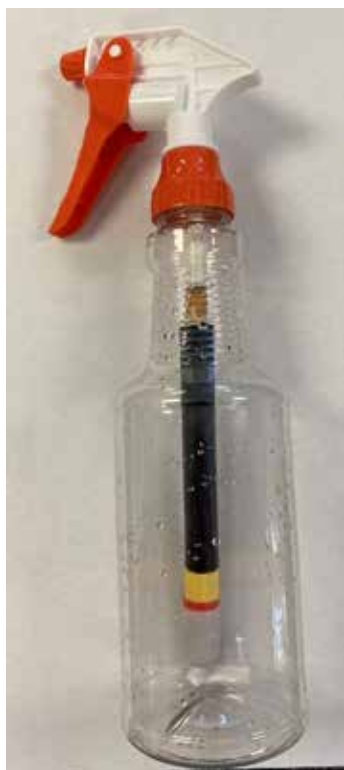
Figure 1: The spray bottle with insert used throughout testing. The bottle was filled with de-ionized water and the spray effluent was collected for use in testing.
