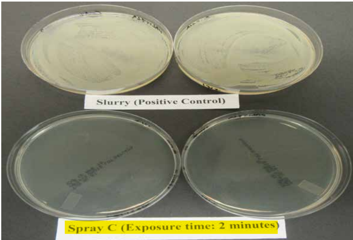
Fig 8: Spray C against bacteria mixture (slurry). Top (positive control); Bottom (treated with the spray C for 2 minutes).
